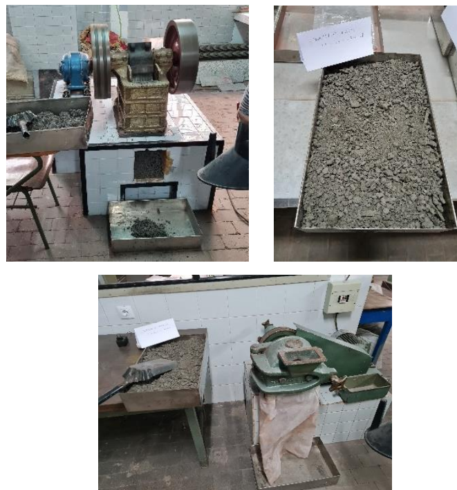
Figure 4-5. Grinding treatment of the La Matona sample
