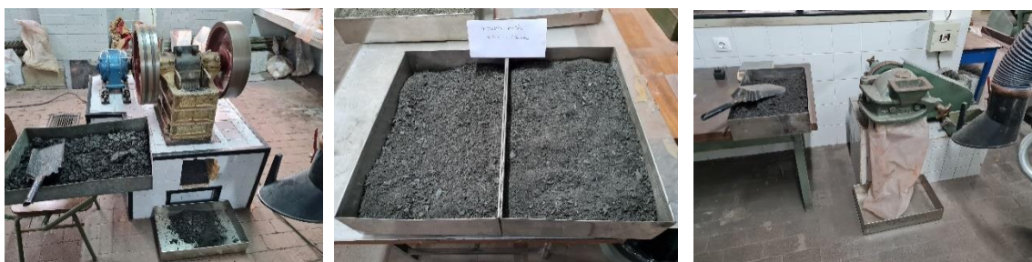
Figure 4-8. Grinding treatment of the El Batán sample
