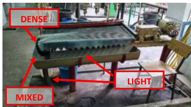
Figure 12-3. Exit areas of the different fractions of the shaking table
