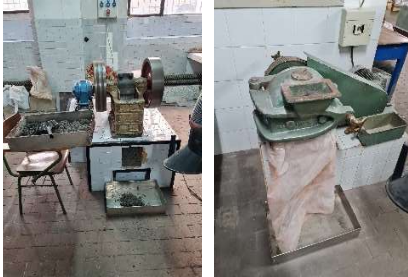
Figure 2-1. Single acting jaw crusher and Disc mill
