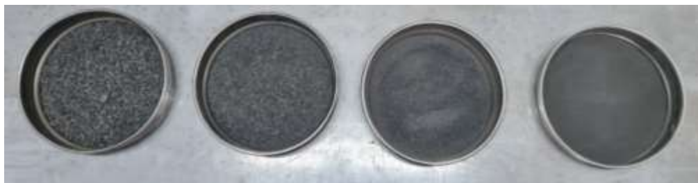
Figure 4-10. Particle size fractions in the sieves, >2.0 mm (left), 2.0-0.5 mm, 0.5-0.1 mm and <0.1 mm (right)
