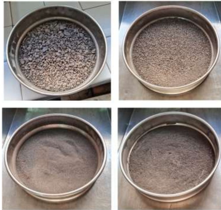
Figure 4-3. Sieve granulometric fractions, >2.0 mm (upper left), 2.0-0.5 mm (upper right), 0.5-0.1 mm (lower left), and <0.1 mm (lower right)
