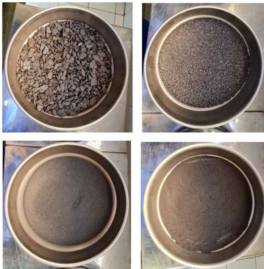
Figure 4-7. Sieve granulometric fractions, >2.0 mm (upper left), 2.0-0.5 mm (upper right), 0.5-0.1 mm (lower left), and <0.1 mm (lower right)
