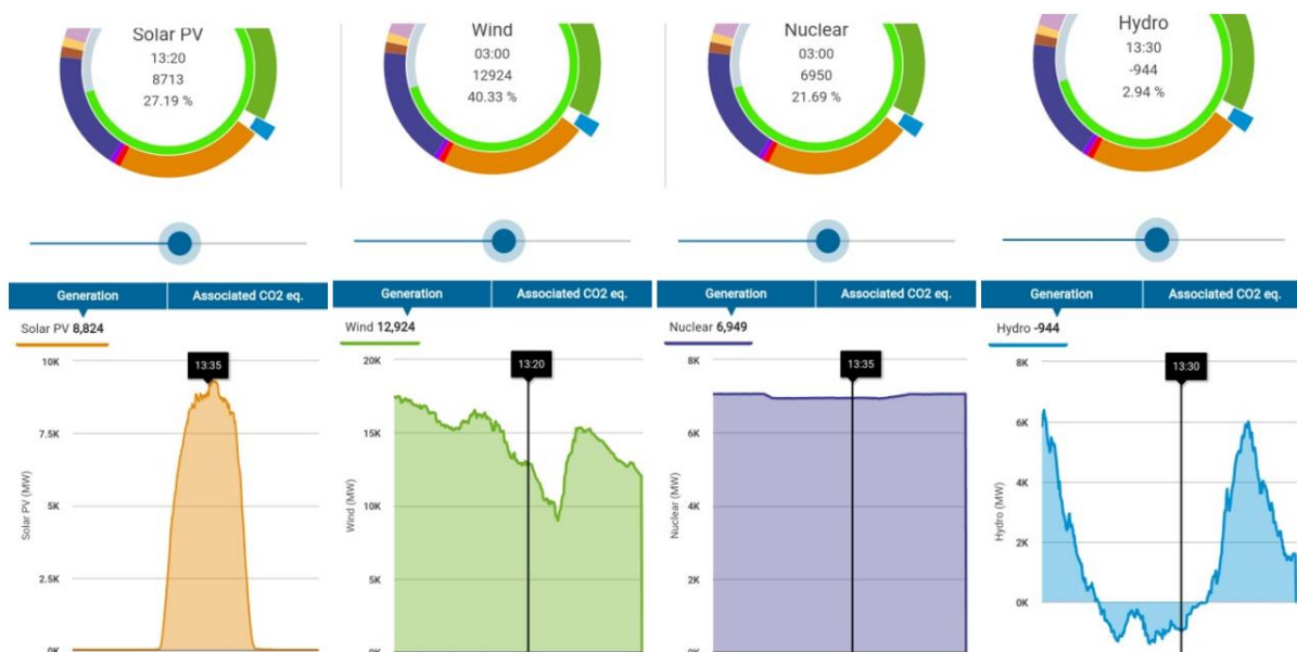
Figure 2-5. Hourly generation patterns of the main emissions-free technologies in the Iberian market (OMIE 2023).
