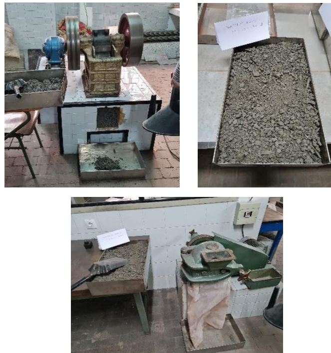
Figure 4-5. Grinding treatment of the La Matona sample
