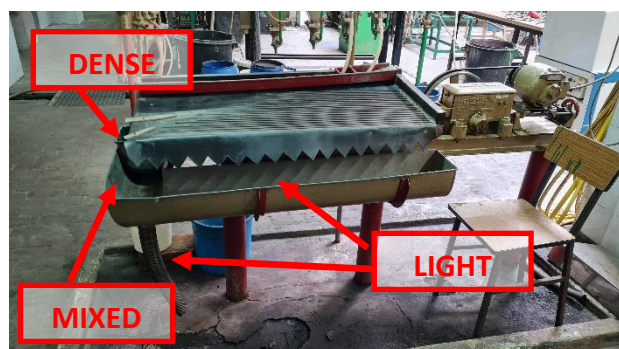
Figure 12-3. Exit areas of the different fractions of the shaking table
