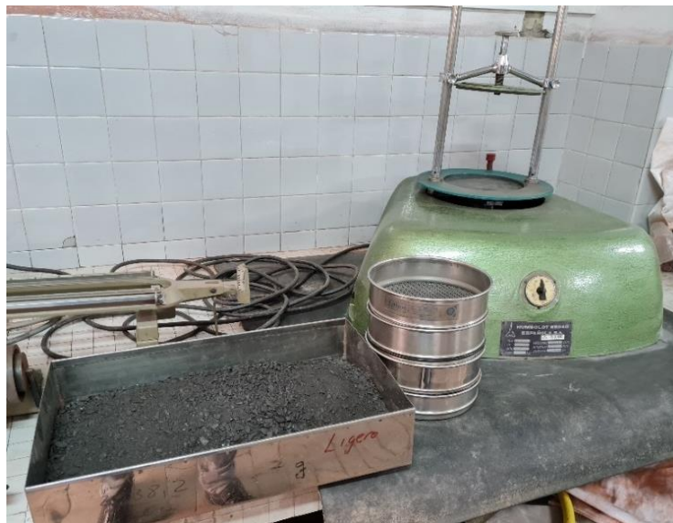
Figure 4-6. Sample of El Batán next to the sieve
