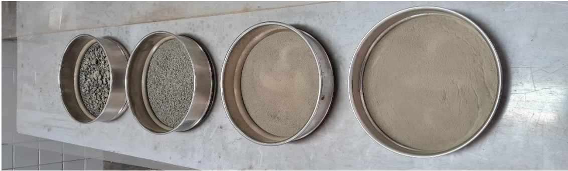
Figure 4-13. Particle size fractions in the sieves, >2.0 mm (left), 2.0-0.5 mm, 0.5-0.1 mm and <0.1 mm (right)
