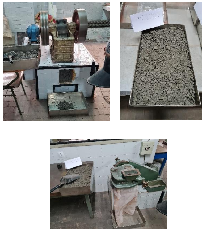
Figure 2-5. Grinding treatment of the La Matona sample
