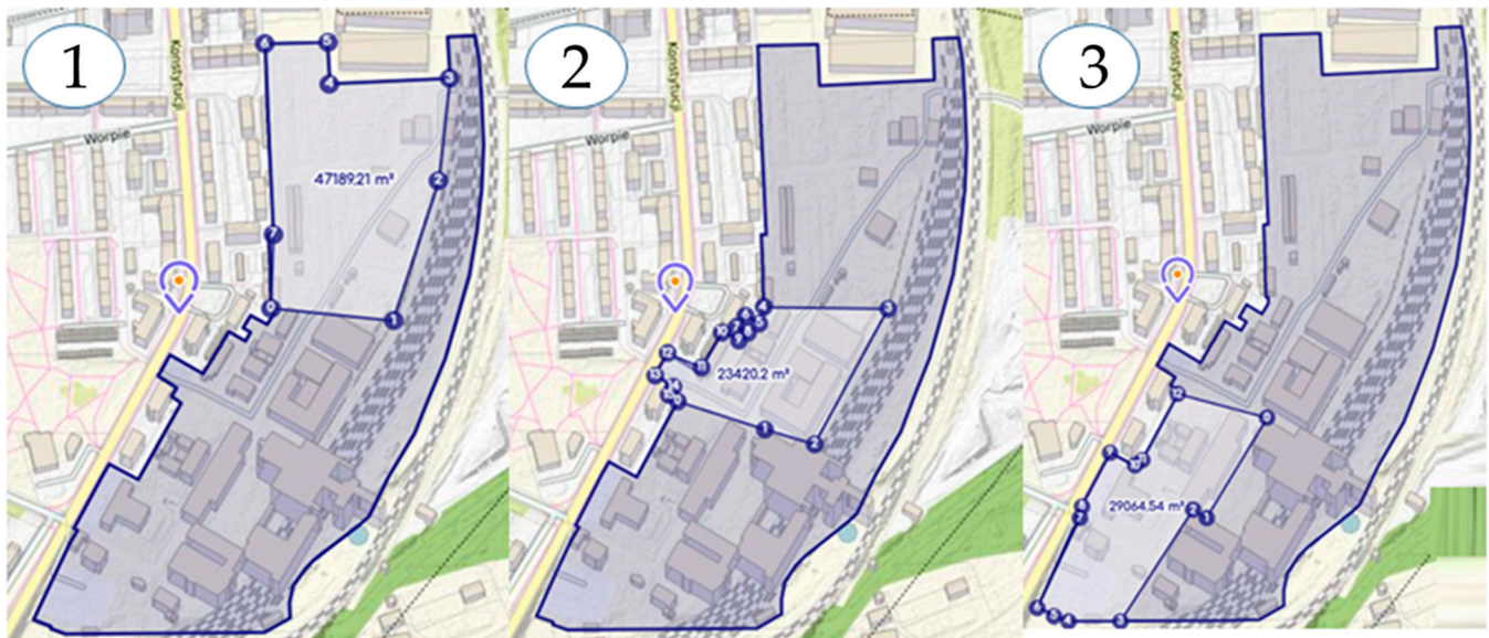
Figure 5. Spatial layout of the three functional areas of the industrial eco-park: (1) a photovoltaic (PV) end-of-life treatment line of 4.72 ha, (2) a central transport and manoeuvring zone of 2.34 ha, and (3) e-waste and household refrigeration-appliance recycling of 2.91 ha.
